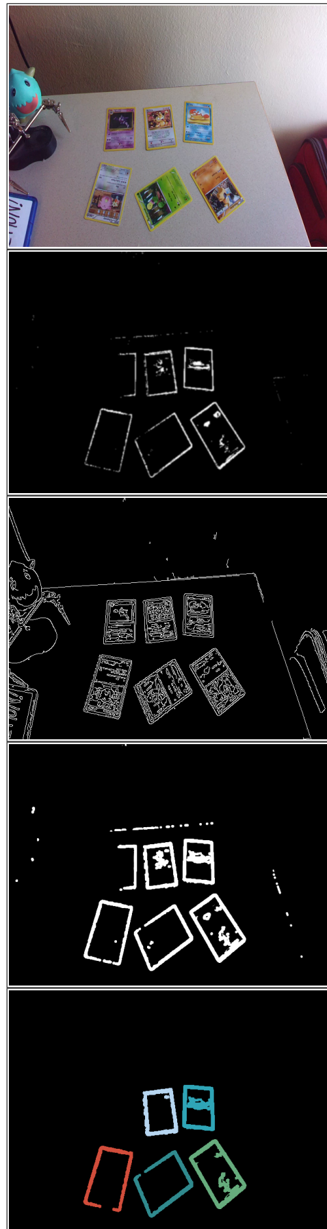
Fig. 3. Sample run of detection pipeline. From top to bottom : original image, color-filtered image, edge-map, "border-map", filtered connected components. (each color represents a different component)
