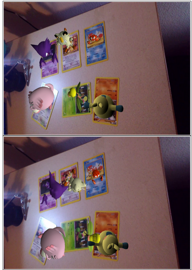
Fig. 7. An example of pose ambiguity; both images represent correct mathematical solutions to the pose estimation problem .
