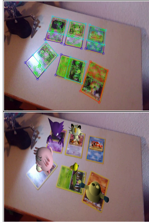
Fig. 10. An example of the tracker showing robustness to glare. (bottom left card) .
