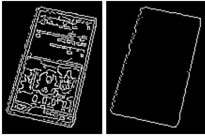
Fig. 5. Sample product of the edge map border filter. Left : original edge map. Right : border-filtered edge map .
