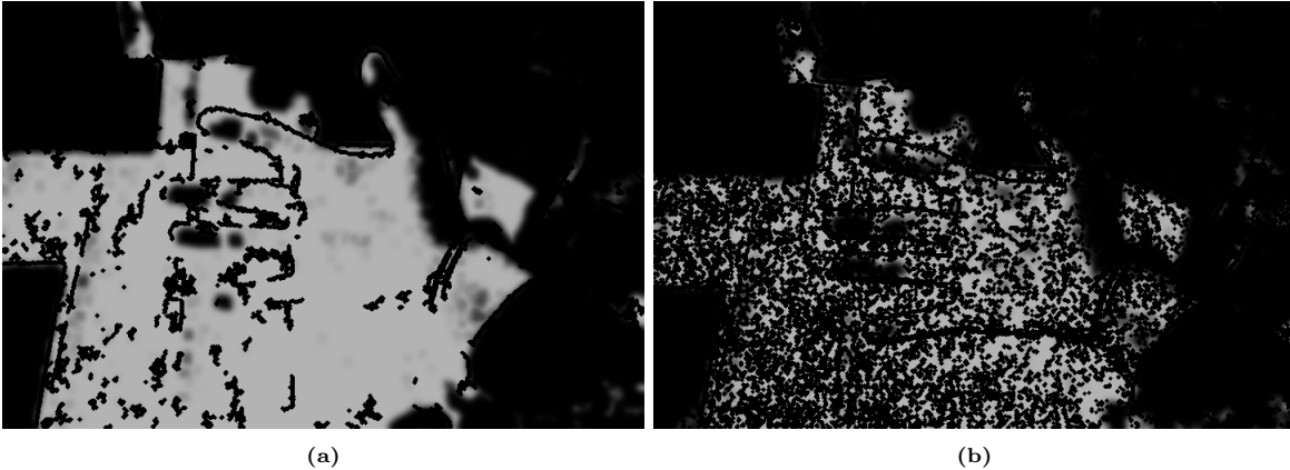
Figure 12: Example of attempts to augment back-projection probabilities for a given image with edge contours detected from RGB space (grayscale was also tried, to no avail). We used edges detected from RGB colorspace for a given image to draw 0-valued contours on top of the back-projection probabilities, which would ideally prevent convex hulls from being created through the edges of the hand. However, we found that either (1) gaps existed between edge contours, precluding forming perfectly-segmented convex hull regions, as in (a); or (2), too many edges were detected as in (b); though a rather extreme example), causing only very small convex hulls to be formed, usually along only a small portion of the hand.
